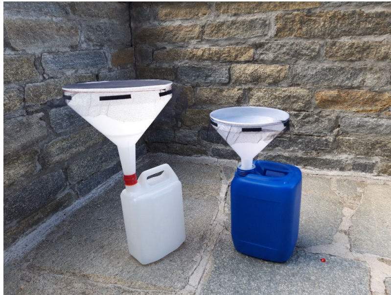
Figure 3. Rain sample collectors. On the left is the collector for chemical analyses; on the right is the collector for isotopic analyses, to which a film of paraffin was added.
