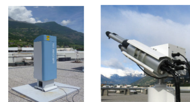
Figure 4. The Advanced Lidar Ceilometer (left) and the aerosol sun photometer (right).
