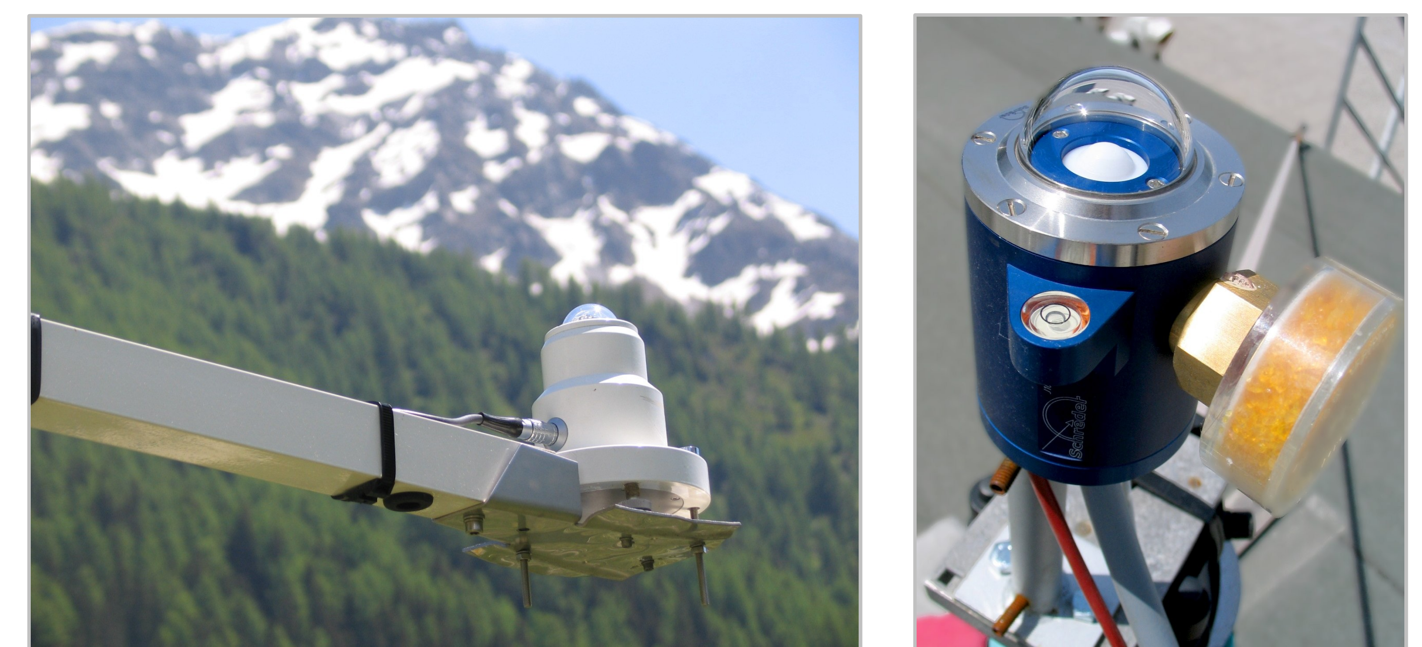
Fig. 7 – A broadband UV radiometer (left) and the diffuser of the Bentham spectroradiometer (right), used by ARPA Valle d'Aosta.
