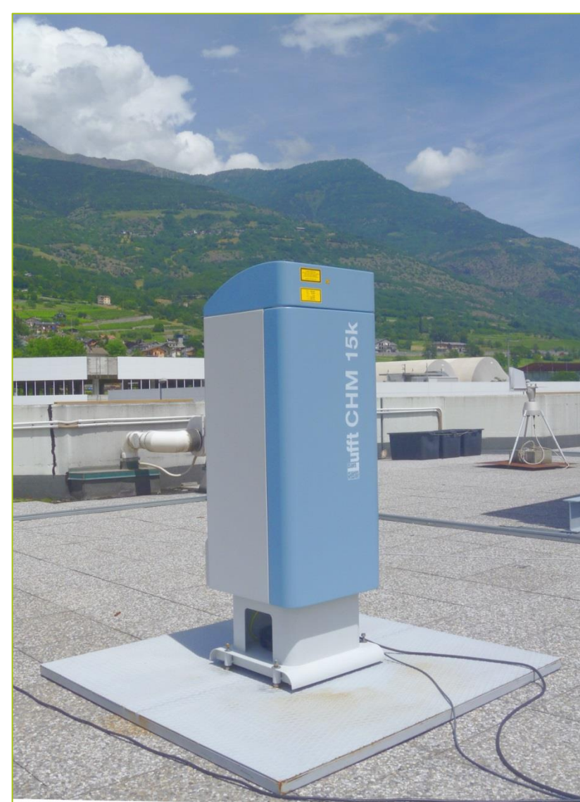
Figure 1: Lufft CHM-15k Nimbus ceilometer.
