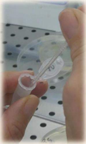
Pre-arricchimento in BPW per 18-24h a  $37^{\circ} \text{C} \pm 1^{\circ} \text{C}$
