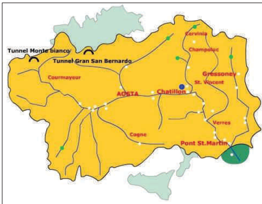
Figure 13 Aosta Valley Water Company HP plants. White dots are run-off hydropower facilities, green dots are dams and reservoirs [taken and modified from the Aosta Valley Water Company website] http://www.cva-ao.it/
