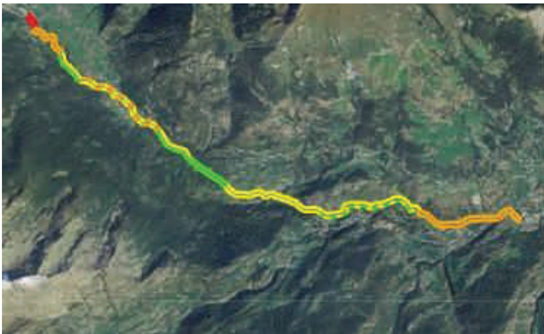
Figure 35 Example of a GIS mapping of IFF values along Dora Baltea river [taken and modified from Gis software].
